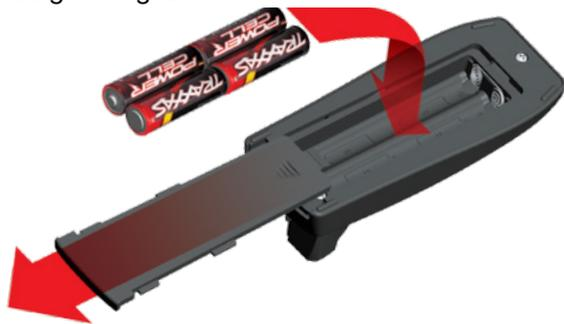
If the status LED flashes red, the transmitter batteries may be weak, discharged, or possibly installed incorrectly. Replace with new or freshly charged batteries. The status LED does not indicate the charge level of the battery pack installed in the model. Refer to the Troubleshooting section on page 11 for more information on the transmitter status LED codes.
