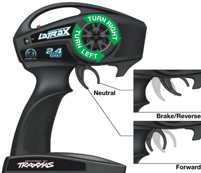
**i** **Using Reverse:** While driving, push the throttle trigger forward to apply brakes. Once stopped, return the throttle trigger to neutral. Push the throttle trigger forward again to engage proportional reverse.
